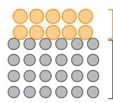
Traditional Concrete Coating (e.g. Epoxy and Polyurethane) "Sticks" to concrete surface via a weak mechanical bond
